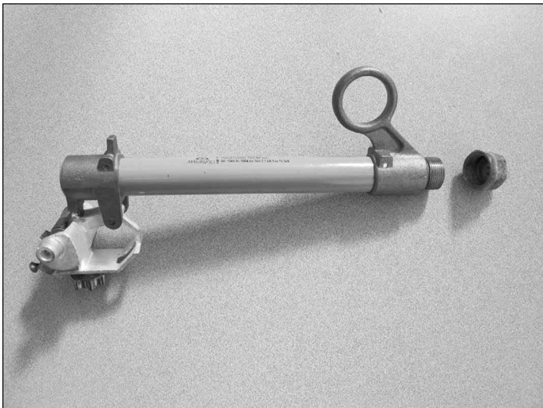
Figure 27: Cutout fuseholder used for the tests.
