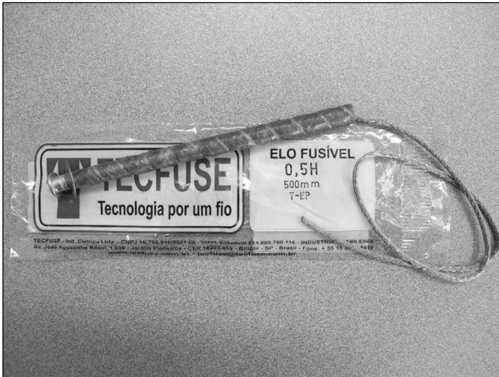
Figure 24: Tested 0.5H fuse link design.
