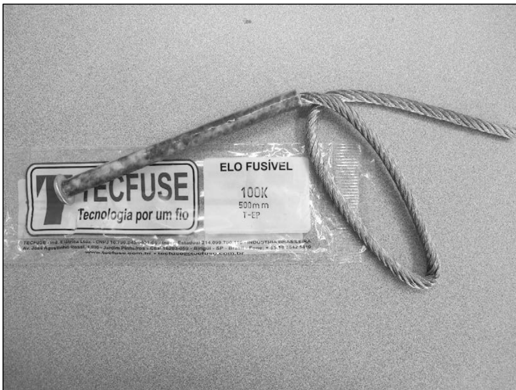
Figure 25: Tested 100K fuse link design.
